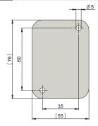
For the positioning of the mounting holes use the housing or the drilling template on page 2.
