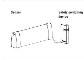
Pressure-sensitive edges are pressure-sensitive protection systems. They are specified in accordance with and meet the requirements of standard EN ISO 13856-2. Pressure-sensitive edges consist of a sensor and a safety switching device
