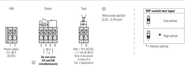
Note: When using the NC outputs (5/6) in Cat. 3 set-up, the wiring with the control must be permanently installed and protected against external damage according to EN ISO 13849-2 Tab.D.4 or else Cat. 2 applies and a test signal is needed.
