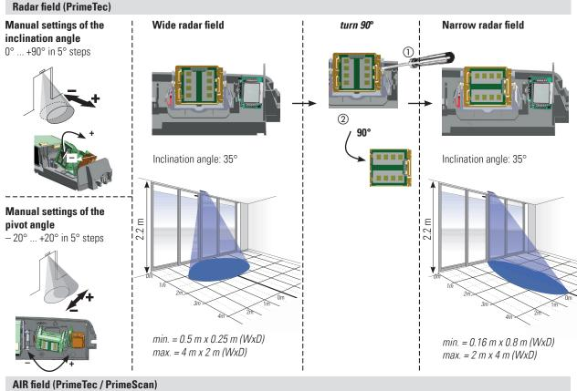
Settings of the inclination angle on the adjustment screw:
