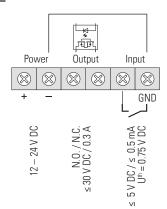
wire cross section: solid  $0.5-1.2~\text{mm}^2$  stranded  $0.3-2.0~\text{mm}^2$
