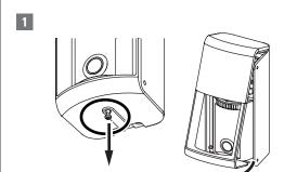
Loosen the retaining screws on the bottom of the front cover and remove the front cover.
