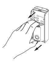
To detach the sensor unit: Hold here and pull forward
