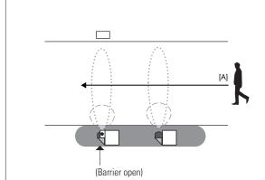
Stand at the edge of the vehicle lane (see figure [B]), walk along the edge and verify that the LED keeps blinking slowly green (not detecting).
