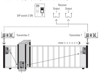
Transmitter input 1 corresponds to receiver output 1 Transmitter input 2 corresponds to receiver output 2
