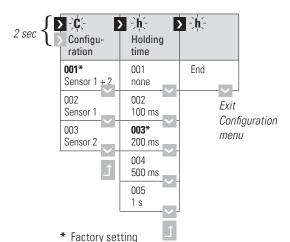
On initial commissioning, the device must be adapted (configured) to the application.
